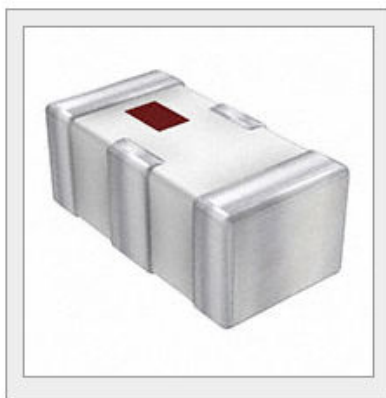
Figure 1 - RF Filter in a Single 0402 Package
