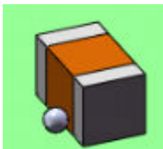
Figure 26 - Solder Ball on a Passive Package
