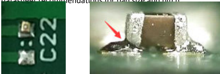
Figure 23 - Example of a Tombstone Defect (left) and an Open Circuit Defect (Right)
